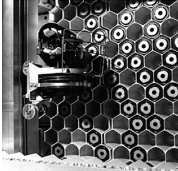
Bild 41: IBM 3851 Storage Compartments
